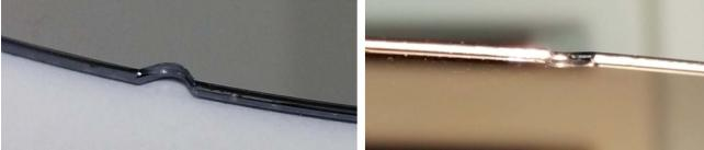
Figure 11. A bonded stack with device wafer thinned to 60  $\mu\text{m}$ .
