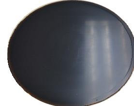
Figure 9. Molded resin wafer with Z-Coat 211 sacrificial layer on silicon carrier.
