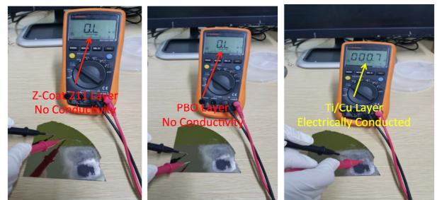
Figure 13. Electrical testing to identify each layer
