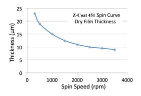
Recommended thickness for bonding is  $15^25$  µm (at  $500^1000$  rpm spin speed).
